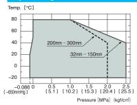
Use after confirmation that the maximum operation pressure and maximum service temperature are within the operation range.
